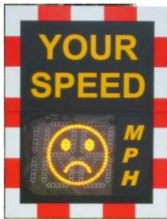
OSPC have two Speed Indicator Devices (SID), which record the number of vehicles travelling over the 30mph speed limit as they pass. Along London Road we have recorded in excess of 100,000 speeding vehicles per month and in one month Passenham Lane had over 20,000 vehicles travelling at speeds in excess of 35mph. The Parish Council are looking to improve the equipment that we own to provide more information that can be downloaded and passed to the Police.
